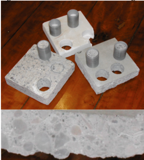
Figure 6. Concrete, limestone and granite used in Cs removal and diffusion experiments.
