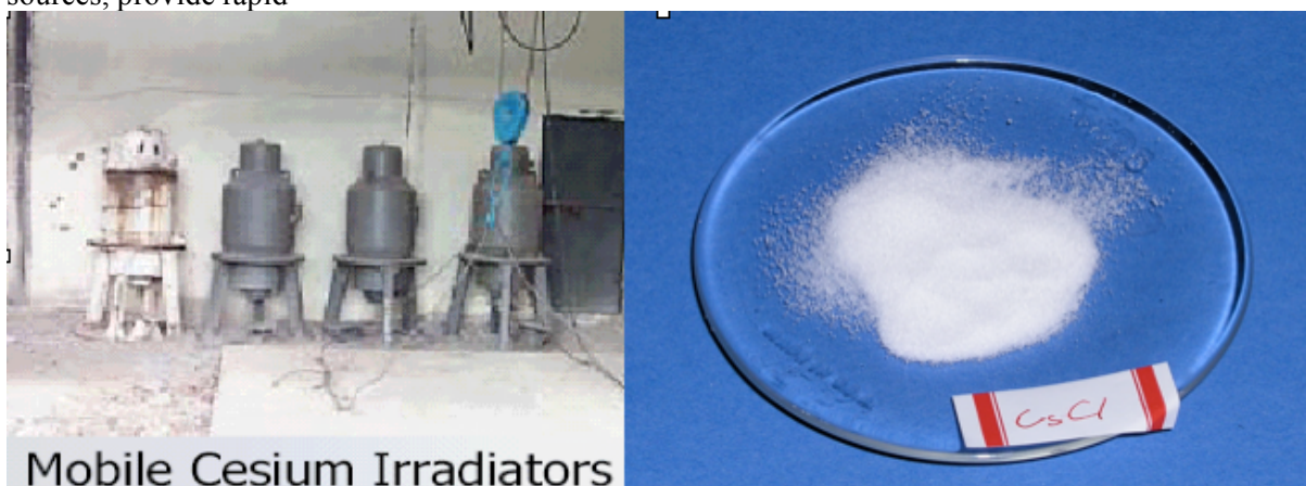
Figure 4. ^{137}\text{CsCl} powder (right) presently used in the irradiation industry. At left are shown abandoned ^{137}\text{CsCl} seed irradiators. ^{137}\text{Cs} emits a hard gamma ray at 0.66 MeV requiring about 18 cm of lead or three feet of concrete to shield. It has a high specific activity (87 Ci/g) and a half-life of 30.17 years, and so must be cleaned up after a ^{137}\text{Cs} dirty bomb attack. In the environment, CsCl dissolves easily into \text{Cs}^+ and \text{Cl}^- . Chemically and biochemically, \text{Cs}^+ behaves like \text{K}^+ and is readily taken up by plants and animals.
